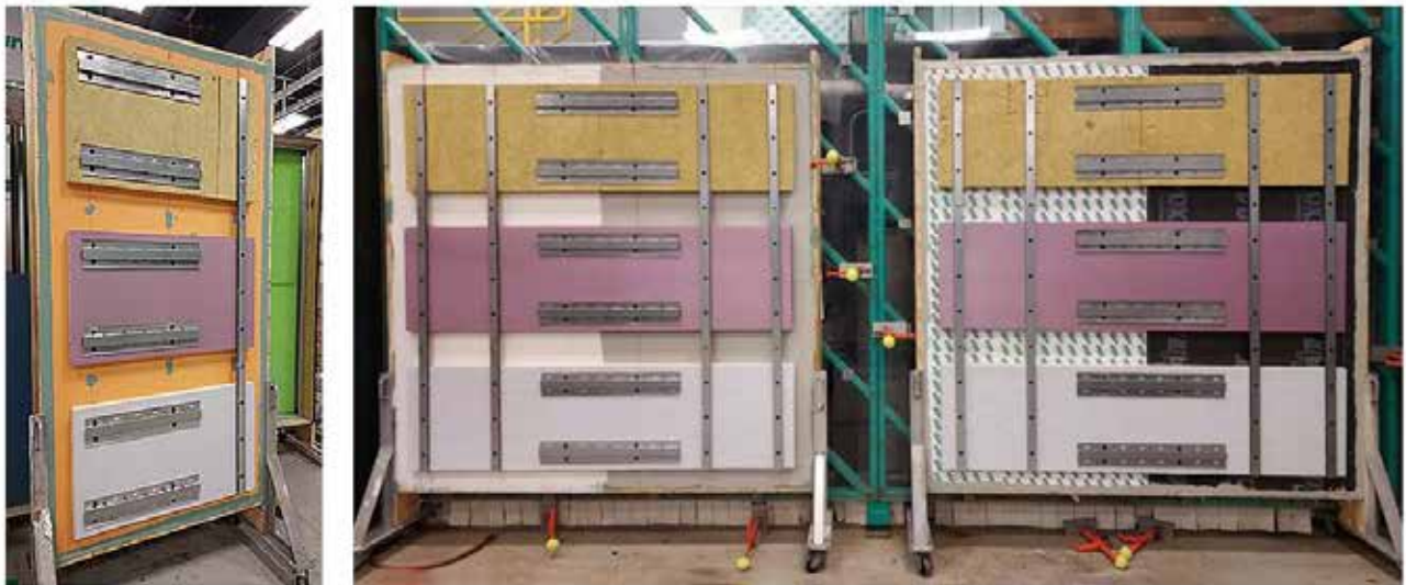
Test walls utilizing various combinations of integrated air barrier sheathing (on left), fluid-applied air barriers (middle) and self-adhered air barriers (right). Note various types of exterior continuous insulation to simulate multiple configurations.
